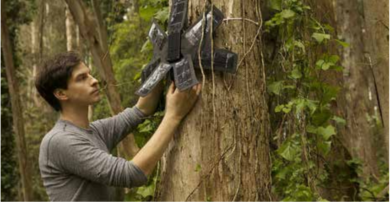
Smartphone devices are hidden in the trees, where they detect sounds of chainsaws (Pic: Rainforest Connection)
