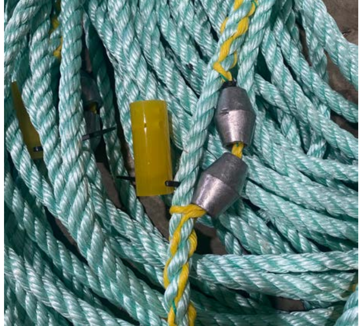
A depth sensor in a yellow plastic protective casing and two barrel weights attached to the floating section of the groundline.
